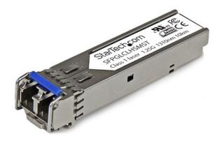
The SFPGLCLHSMST is a Cisco GLC-LH-SM compatible fiber transceiver module that has been designed, programmed and tested to work with Cisco brand switches and routers. It delivers dependable 1GbE (1000 Mbps) connectivity over fiber cable, for 1000BASE-LX/LH compliant networks, with a maximum distance of up to 10 km (6.2 mi).
