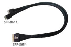
SFF-8654 (host) to SFF-8611 Oculink (device) PCIe 4.0 x8 NVMe cable. Each cable can host up to 2x NVMe SSDs.
