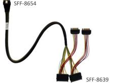
SFF-8654 to U.2 SFF-8639 cable with a 15-pin SATA power connector. Each cable supports two U.2 NVMe SSDs.
