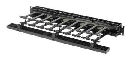
Single Sided Horizontal Managers are available in 1RU and 2RU sizes. The unique finger design protects cables from damage while the cover mounts with six hinge clips to allow the door to be opened one handed without becoming "unhinged". They are designed to mount on any 19" EIA style rack or cabinet.
