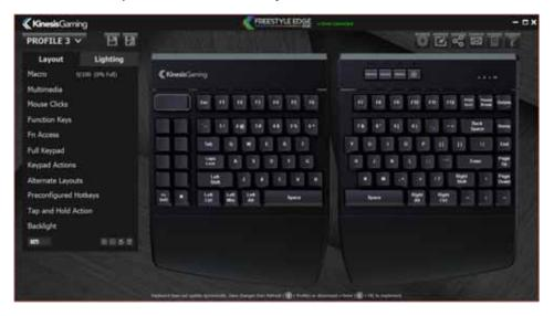
**Navigating Layers**: The "top-layer" action and the "Fn-layer" action can be customized separately. Use the Layer toggle-switch in the Action Menu to move between the layers during programming.
