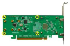
After removing the screws, carefully remove the heat sink from the SSD7502.
