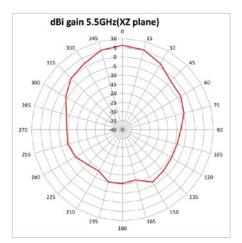
Radiation Pattern for 5GHz Antenna 2
