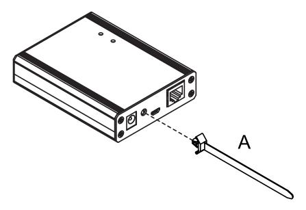
3. Insert the other end of the DC Jack Lock component A through the component B's joint.
