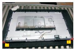
S11 Disconnect the LED cable from the connector of the interface board, then release the LED cable by tearing off the 2pcs tapes.
