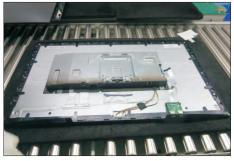
Use a Philips-head screwdriver to remove 2pcs screw for unlocking the key board, then tear off the tapes and release the key board.
