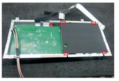
Use a Philips-head screwdriver to remove 7pcs screws for interface board and power board. (No.1 screw size=M4x8, Torque=7±1kgfxcm; No.2~7 screw size=M3x7.5, Torque=7±1kgfxcm)
