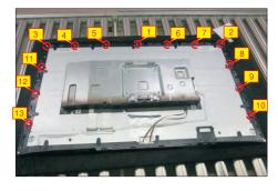
S10 Use a Philips-head screwdriver to remove 2pcs screws for unlocking the middle bezel with the front bezel.
