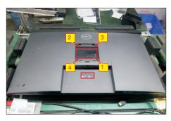
Tear off screen protector, then wedge your fingers between rear cover and the middle bezel on the corners of the top side of the monitor to release the rear cover, then use one hand to press the middle bezel, the other hand to pull up the rear cover in order of arrow preference for unlocking the rear cover.
