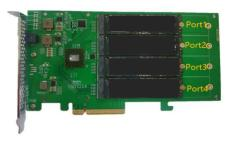
Step 7. Replace the heat sink after installing all SSDsStep 8. On the rear of the SSD7204, refasten the six screws that were removed in step 1.
