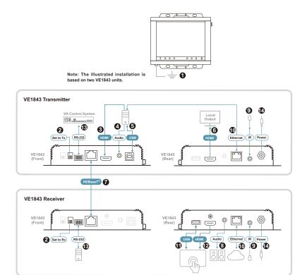
1. Ground the VE1843 by connecting one end of a grounding wire to the grounding terminal and the other end to a suitable grounded object.
