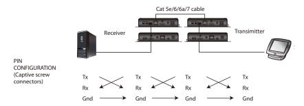
The general concept here is that a RS-232 signal can be transmitted (Tx) to the receiving (Rx) end of a unit. The received signal can then be transmitted (Tx) to the receiving (Rx) end of another unit. The RS-232 signals can be transmitted back the other way.
