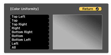
9. Select **Red**, **Green**, or **Blue** and press the left arrow button to weaken the color tone or the right arrow button to strengthen the color tone.
