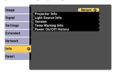
Select **Light Source Info** to display the projector's light source information. Select **Version** to display the projector's firmware version. Select **Temp Warning Info** to display the projector's high temperature warnings. Select **Power On/Off History** to display the projector's power on and off history. Select **Projector Info** to display the settings described below.
