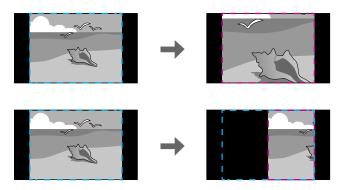
• Full Display to adjust the image to the projector's screen size as you scale the image
