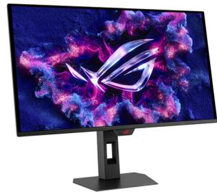
26.5" 2560 x 1440 QD-OLED, 1073.7M, 0.03ms, 500Hz, DisplayPort, HDMI, 65W, 100-240V, 50/60Hz
