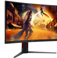
AOC G4 CQ32G4. Display diagonal: 80 cm (31.5"), Display resolution: 2560 x 1440 pixels, HD type: Quad HD, Display technology: LED, Response time: 4 ms, Native aspect ratio: 16:9, Viewing angle, horizontal: 178°, Viewing angle, vertical: 178°. VESA mounting, Height adjustment. Product colour: Black, Red
