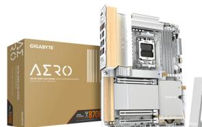
**Product name :** X870E AERO X3D WOOD Motherboard - Supports AMD Ryzen 9000 CPUs, 16+2+2 Phases Digital VRM, up to 9000Hz DDR5 (OC), 2xPCIe 5.0 + 2xPCIe 4.0, Wi-Fi 7, 5GbE LAN, USB 4
