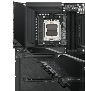
B850 AORUS STEALTH Motherboard - AMD Ryzen 9000 Series CPUs, 14+2+2 Phases Digital VRM, up to 8200MHz DDR5 (OC), 2xPCIe 5.0 + 2xPCIe 4.0 M.2, WIFI 7, 5 GbE LAN, USB 3.2 Gen 2
