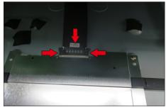
Tear off 4pcs rubbers, then use a Philips-head screwdriver to remove 2pcs screws for unlocking the small bracket with T-Con board, then remove the small bracket, then release the LED key cable by tearing off tapes on the back of the cable.
