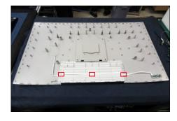
Use a Philips-head screwdriver to remove 7pcs screws for unlocking the two speakers. Release the left speaker cables from the probers of the middle frame, and then disconnect the speaker cable, LED cable and USB cable away from the connector.
