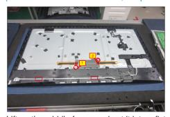
S16 Lift up the middle frame and put it into a fixture, tear off the maylar tape for releasing the LED key board away from the middle frame.
