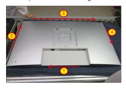
Lift the rear cover up carefully. Disconnect the joystick key cable from the connector of the interface **S6** board, and then remove the rear cover and put it aside for later disassembling.
