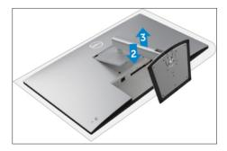
Use a Philips-head screwdriver to remove 4pcs screws for unlocking mechanisms. Remove DP caps. **S4** (No.1~4 screw size=M4x11; Torque=11±1kgfxcm)
