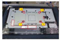
S14 Lift up the bracket chassis, and disconnect the LVDS cable from the connector of the T-CON board of panel module, then put the bracket chassis on a protective cushion for later disassembling.
