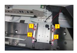
Use a Philips-head screwdriver to remove 2pcs screws for unlocking the USB cover, remove the USB cover, then use a Philips-head screwdriver to remove 1pcs screw for locking the USB board with the USB bracket. Disconnect the USB connective cable.
