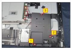
Use a Philips-head screwdriver to remove 4pcs screw for unlocking the USB unit with the middle frame, and then release the USB unit from the hooks of middle frame.
