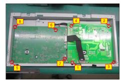
Remove the circuit boards from the bracket chassis module carefully, and then disconnect all of the cables.
