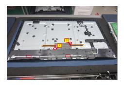
S14 Lift up the middle frame and put it into a fixture, tear off the maylar tape for releasing the LED key board away from the middle frame.
