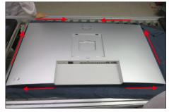
Use a Philips-head screwdriver to tighten four screws for locking mechanisms. Paste 1pcs label on the specific positions as the picture below shown.
