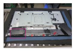
Tear off 1pcs aluminum foil to release the bracket chassis. Use a Philips-head screwdriver to remove 28pcs screws for unlocking the middle frame with the panel module.
