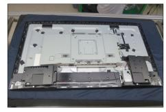
Use a Philips-head screwdriver to remove 2pcs screw for unlocking the joystick board, then tear off the tapes and release the joystick board.
