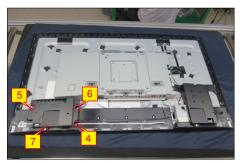
Take 1pcs joystick key, 1pcs joystick board and 1pcs rear cover, then assemble the joystick key with the board, then paste 1pcs conductive foam on the back of the board. Locate the joystick board to the correct position of the rear cover, then use a Philips-head screwdriver to lock 2pcs screws for locking the joystick board with rear cover. Tear off the papers on the back of the cable, and then fix the joystick cable with tapes.
