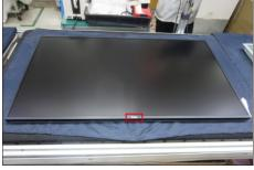
Turn over the panel module to place screen faced down. Paste 2pcs shading tape on the left and right side of the panel corner, then paste 27pcs acetate tapes on the specific position of the back of panel as the picture below shown.
