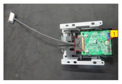
Release the speakers' cable to from the hooks of the middle frame, then remove the speakers.
