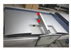
Use a protective bag to pack the stand base, then lift up the monitor to checking the gap between the front bezel with panel module, then provide power supply and a video signal to the monitor, then turn on the monitor for functionality check.
