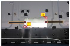
Move the bracket chassis module close to the panel module, then connect the LVDS cable to the S10 connector of the T-Con board, then put the bracket on the back of the panel module.
