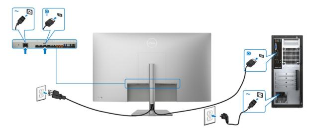
4. How to connect and disconnect power cable/ connectivity cable
