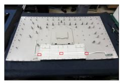
Move the assembled rear cover close to the panel unit, then connect the joystick key cable to the connector of interface board. Put down the rear cover and push the rear cover on the positions marked as the picture below shown for mechanisms engagement.
