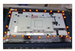
S11 Tear off 3pcs aluminum foil, then use a Philips-head screwdriver to remove 4pcs screws for locking the bracket chassis module with the panel.
