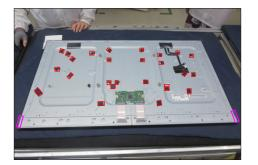
Use a Philips-head screwdriver to remove 9pcs screws for unlocking power board and interface board with the bracket.
