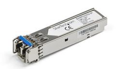
The EW3P0000559-ST is a Citrix EW3P0000559 compatible fiber transceiver module that has been designed, programmed and tested to work with Citrix brand switches and routers. It delivers dependable 1 GbE connectivity over fiber cable, for 1000BASE-LX compliant networks, with a maximum distance of up to 10 km (6.2 mi).
