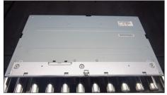
Remove the Mylar tape from the hooks of the bracket chassis.
