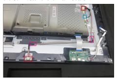
Take a pair of speakers to locate the probers, then Use a Philips-head screwdriver to tighten 6pcs screws for locking the two speakers with the middle frame, and then connect the speaker's cable to the connector of the main board and fix the cables and with 3pcs acetate tape as the picture below.
