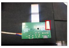
Locate the USB board into the hook of the middle frame. Use a Philips-head screwdriver to tighten 1pcs screw for locking the USB unit with the middle frame, then connect the two USB cables to the connectors of main board, then fix the cable with 1pcs aluminum foil as the picture below shown. (No.1 screw size=M3x3.5, Torque=4±0.5 kgfxcm)
