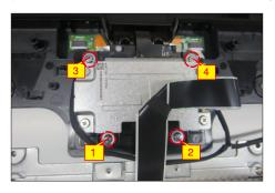
Use a Philips-head screwdriver to remove 4pcs
