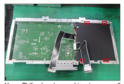
Use a Philips-head screwdriver to remove 8pcs screws for interface board and power board with the bracket chassis module.
