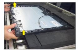
Use a Philips-head screwdriver to remove 4pcs screws for unlocking the left and right Mic boards with the middle frame, then release the two Mic boards away from the middle frame.
