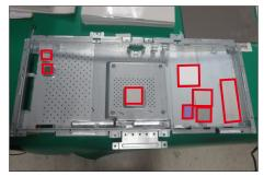
S2 Turn over a power board and put the power board into the bracket chassis, settle the panel power cable to the correct position.
