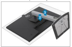
Use a Philips-head screwdriver to remove 4pcs screws for unlocking mechanisms. Remove DP cap.
