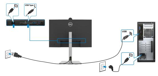
4. How to connect and disconnect power cable/ connectivity cable
