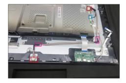
Tear off 1pcs aluminum foil for releasing the USB cable. Use a Philips-head screwdriver to remove 1pcs screw for unlocking the USB unit, then disconnect the two USB cables away from the connectors of interface board. Release the USB board away from the hook of the middle frame.
