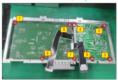
Remove the power board and interface board from the bracket chassis module carefully, and then disconnect all of the cables.
