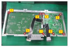
Turn over the bracket chassis, and then take 1pcs black mylar to insert the hooks of the bracket chassis to cover the power board.
