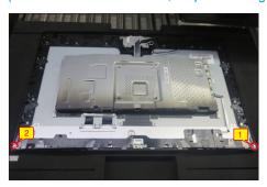
Use a Philips-head screwdriver to remove 4pcs screws for unlocking the camera unit.
