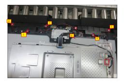
Disconnect the panel lamp cable away from the interface board and panel module, then tear off the tape and remove the panel lamp cable. Disconnect the camera cable away from the connector of the interface board.
