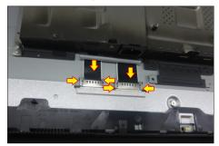
Use a Philips-head screwdriver to tighten 4pcs screws for locking the bracket with the panel, then take 1pcs camera cable to connect camera with main board.
