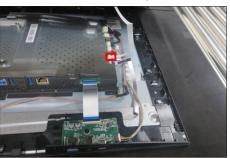
Use a Philips-head screwdriver to remove 3pcs screw for unlocking the joystick board, then tear off all the tapes and release the joystick cable.
