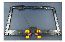
Tear off the release paper on the back of the touch cable and then fix the cable on the back of the panel.
