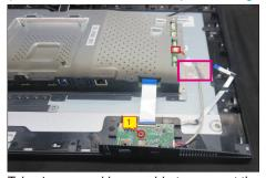
Take 1pcs panel lamp cable to connect the main board with panel, then fix the lamp cable on the back S18 of the panel with tape. Connect the camera cable to the connector of the main board.
