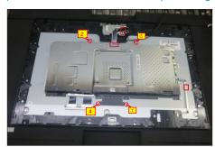
S13 Disconnect the LVDS cables away from the connectors of the panel module, then lift up and take away the bracket chassis and put it on a protective cushion.
