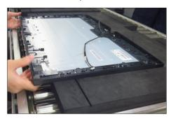
Use a Philips-head screwdriver to lock 13pcs screws for locking the middle frame unit with the panel, then paste 2pcs aluminum foil to fix the Mic board.
