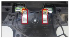
Take 1pcs camera unit assembled in LCM line, then locate the camera unit into the pins of the middle frame.
