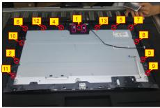
S16 Lift up the middle bezel away from the pane module, then put it on a cushion foam for later disassembling.
