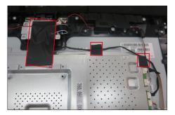
connect the touch cable to the connector of the interface board, then paste 2pcs aluminum foil on S20 the specific positions for fixing the bracket and panel connectors as the picture below shown.
