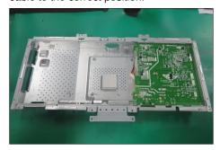
Take 1pcs interface board, connect 2pcs LVDS cable to the connectors of the interface board, then connect the cable of the power board to the connector of the interface board. Turn over the interface board and locate it into the main chassis. Use a Philips-head screwdriver to tighten 8pcs screws for locking the interface board and power board.
