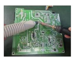
S24-5 Lift the bulk cap. up and away from the PCB.
