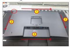
S6 Lift the rear cover up carefully. Disconnect the joystick key cable from the connector of the main board, and then remove the rear cover and put it aside for later disassembling.
