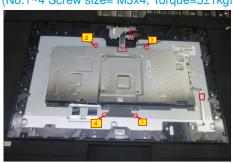
Disconnect the LVDS cables away from the connectors **S15** of the panel module, then lift up and take away the bracket chassis and put it on a protective cushion.
