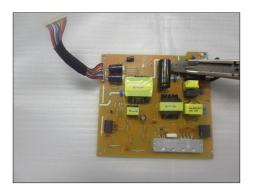
S24-4 Take out bulk cap. pin solder with soldering iron and absorber.
