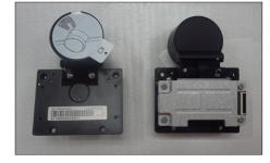
Tear off 2pcs aluminum foil to release the Mic boards Use a Philips-head screwdriver to remove 13pcs
