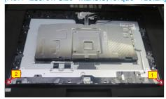
Use a Philips-head screwdriver to remove 4pcs screws for unlocking the camera unit.
