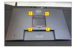
Wedge your fingers between rear cover and the middle bezel on the corners of the top side of the monitor to release the rear cover, then use one hand to press the middle bezel, the other hand to pull up carefully the rear cover in order of arrow preference for unlocking mechanisms of rear cover.
