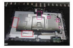
Tear off 3pcs acetate tapes, then disconnect the speakers' cable away from the connector of the main board, and then use a Philips-head screwdriver to remove 6pcs screws for unlocking the two speakers with the middle frame, and remove the speakers.
