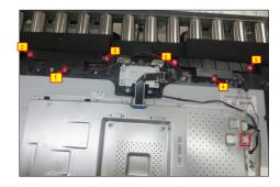
S10 Disconnect the panel lamp cable away from the interface board and panel module, then tear off the tape and remove the panel lamp cable. Disconnect the camera cable away from the connector of the interface board.
