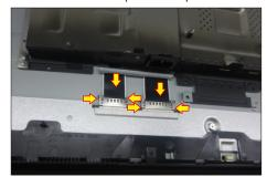
Release the assembled camera unit from the S16 probers of the middle frame and put it aside for later disassembling.
