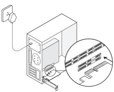
c. Replace the case panel, plug in the power cable and turn on your computer. Then connect the Ethernet cable to the adapter.
