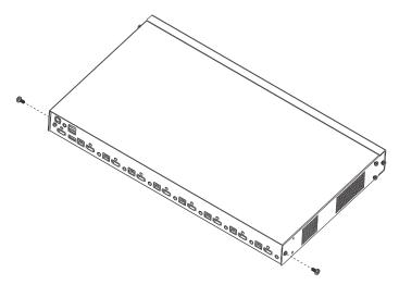
2. Use the M3 x 8 Phillips hex head screws supplied with the rack mounting kit to screw the rack mounting brackets into the sides near the rear of the unit.
