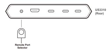
Prepare a USB Type-A to Type-C cable. Connect one end of the USB Type-A cable to the computer and the other end to the US3310 USB 3.2 Gen 1 Type-C Port 1.
