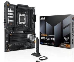
AMD AM5, AMD X870, 4 x DIMM slots, max. 192GB, DDR5, 1 x Realtek 2.5Gb Ethernet, 2x2 Wi-Fi 7 (802.11be), 256 Mb Flash ROM, UEFI AMI BIOS, ATX
