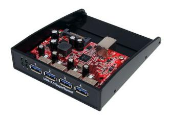
The 35BAYUSB3S4 3.5-inch Front Bay to 4-Port USB 3.2 Gen 1 Panel Hub is TAA compliant and turns any available 3.5-inch computer case front bay into a 4-Port USB 3.2 Gen 1 hub.
