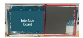
Unlock 10 PCBA screws to disassemble "Interface board", "Power board" and "LED Driver board" from "Main Shielding"
