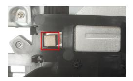
S11 Insert 2 "USB board FFC" and 1 "USB board Wire" into "USB board"
