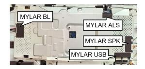
S16 Assemble "Speaker" to "Middle Frame" and fix it by screw\*6 (See yellow mark)
