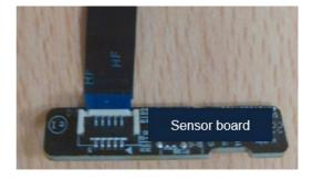
S14 Assemble "Sensor board" into "Middle Frame"
