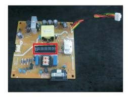
S20-1 Cut the glue between bulk cap. and PCB with a knife.
