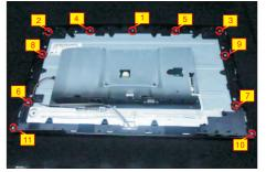
S11 Disconnect the LED cable from the connector, then release the LED cable by tearing off 2pcs tapes.
