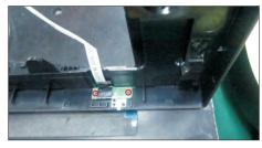
S13 Lift up the panel with the bracket for releasing the front bezel away from the panel. Use a Philips-head screwdriver to remove one screw for unlocking the bracket with panel.
