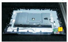
Tear off 2pcs aluminium foils for unfixing the bracket.
