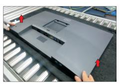
S6 Lift the rear cover up carefully. Disconnect the key cable and USB FFC cable from the connectors of the interface board, and then remove the rear cover.
