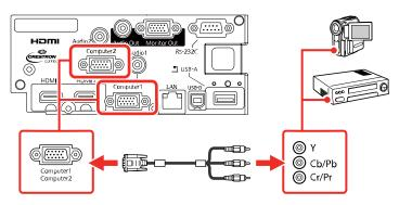
3. Tighten the screws on the VGA connector.
