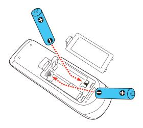
**Warning:** Make sure the batteries are inserted in the correct positions. If the batteries are not inserted correctly, they could explode or leak, causing a fire, injury, or damage to the product.
