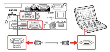
4. Tighten the screws on the VGA connector.
