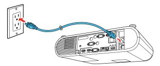
2. Plug the power cord into an electrical outlet.
