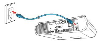
**Caution:** To avoid damaging the projector or lamp, never unplug the power cord when the status light is on or flashing.
