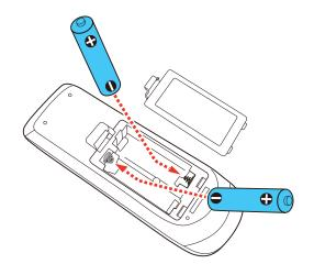
**Warning:** Make sure the batteries are inserted in the correct positions. If the batteries are not inserted correctly, they could explode or leak, causing a fire, injury, or damage to the product.
