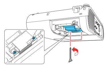
6. Grasp the raised section of the lamp and gently pull the lamp out of the projector.
