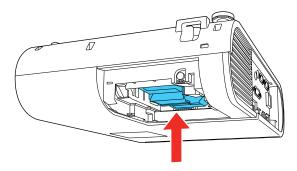
Caution: Do not touch any glass on the lamp assembly to avoid premature lamp failure.
