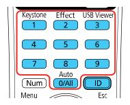
4. Press the ID button on the remote control to check if the ID-setting process worked.
