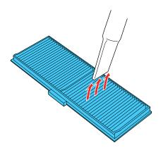
**Note:** If dust is difficult to remove or the air filter is damaged, replace the air filter.
