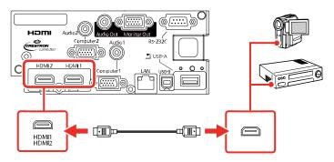
**Note:** If you have problems hearing audio through the HDMI connection, you can use one of the projector's audio ports instead to play sound. Connect one end of an optional 3.5 mm stereo mini-jack audio cable to one of the projector's audio ports and the other end to your video source's audio out port. Then select the audio port you connected to as the **HDMI1 Audio Output** or **HDMI2 Audio Output** setting in the Extended menu.
