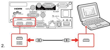
**Note:** If you have problems hearing audio through the HDMI connection, you can use one of the projector's audio ports instead to play sound. Connect one end of an optional 3.5 mm stereo mini-jack audio cable to one of the projector's audio ports and the other end to your computer's audio out port. Then select the audio port you connected to as the **HDMI1 Audio Output** or **HDMI2 Audio Output** setting in the Extended menu.
