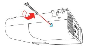
**Warning:** If the lamp is broken, glass fragments may be loose inside the lamp chamber. Be careful removing any broken glass to avoid injury. If the projector is installed on the ceiling, stand to the side of the lamp cover and not underneath it; pieces of glass could fall into your eyes or mouth when you open the lamp cover.
