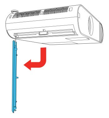
3. Pull the air filter out of the projector.
