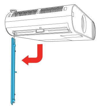
4. Pull the air filter out of the projector.
