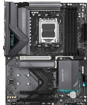
**GIGABYTE X870 EAGLE WIFI7 Motherboard - Supports AMD Ryzen 9000 CPUs, 14+2+2 phases VRM, up to 8000MHz DDR5 (OC), 1xPCIe 5.0 + 2xPCIe 4.0, Wi-Fi 7, 2.5GbE LAN, USB 4:**
