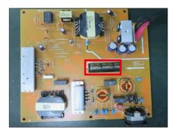
S23-1 Cut the glue between bulk cap. and PCB with a knife.
