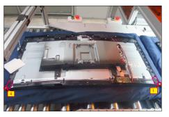
Use a Philips-head screwdriver to remove 1pcs screw for unlocking the USB board, then disconnect the USB cable and touch cable away from the connectors of main board. Release the USB board away from the hook of the middle frame. (No.1 screw size=M3x3.5, Torque=4±0.5 kgfxcm)
