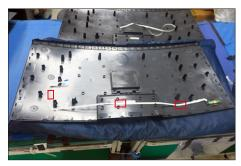
Tear off 2pcs tape, then disconnect the LED cable away from the connector of the interface board. Use a Philips-head screwdriver to remove 2pcs screws for unlocking the middle frame and front frame. (No.1~2 screw size=M2x3.3,Torque=1±0.2kgfxcm)
