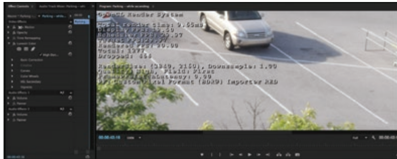
Figure 4. Premiere Pro has a display mode that monitors display FPS and dropped frames. To access, click Ctrl+Shift+F11.
