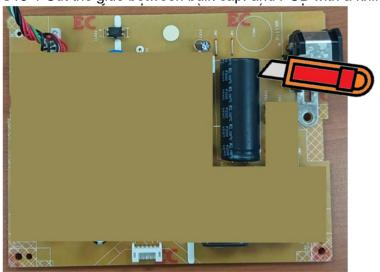
S18-2 Ensure cutting path within the glue, don't touch bulk cap. or PCB
