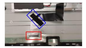
S13 Unlock 13 screws to disassemble "Middle Frame" from "Panel"
