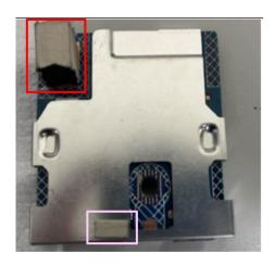
S10 Disassemble "USB board" from "USB Shielding"
