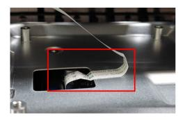
S6 Unlock 3 screws to disassemble "Control board" from "Rear Cover"
