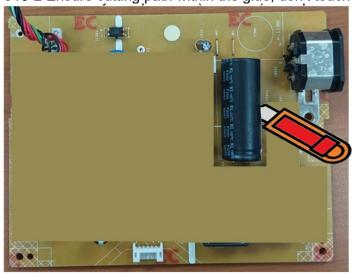
S18-3 Take out bulk cap. pin solder with soldering iron and absorber
