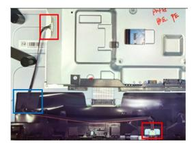
S9 Assemble "USB board" with "USB Shielding"
