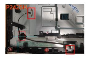
Assemble "USB board" with "USB Shielding"
