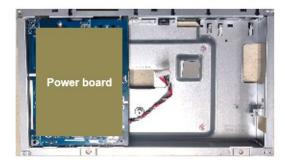
S2 Insert "LVDS FFC" into "Interface board"
