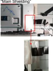
Tear off a black tape from "USB board FFC" and "Panel
