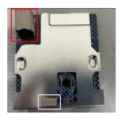
S11 Disassemble "USB board" from "USB Shielding"
