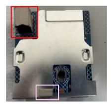
S12 Assemble "USB board" with "Middle Frame"
