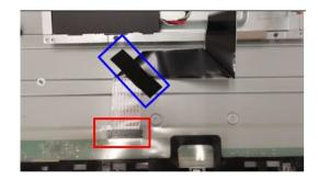
S15 Unlock 13 screws to disassemble "Middle Frame" from "Panel"
