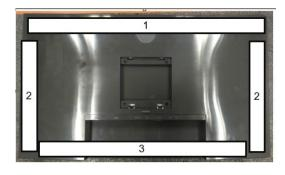
Pull out "Control board FFC" from "Interface board" and tear off it from "Main Shielding" to take off "Rear Cover"
