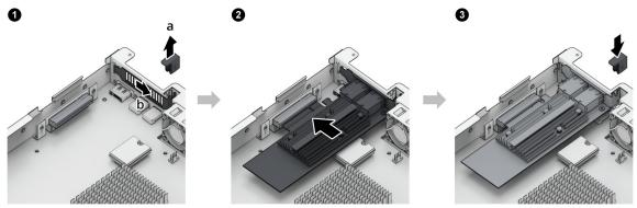
**Note:** Confirm that the network interface card is fully inserted. Otherwise, the network interface card might not be able to function properly.
