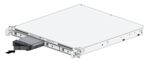
Note: Make sure that the drive tray is completely inserted. Otherwise, the drive might not function properly.
