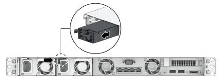
4 Prepare a new PSU. Insert it into the empty slot until you hear a click.
