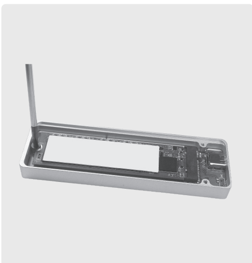
5. Insert the screw thru the Spacer and fasten onto the M.2 holder.
