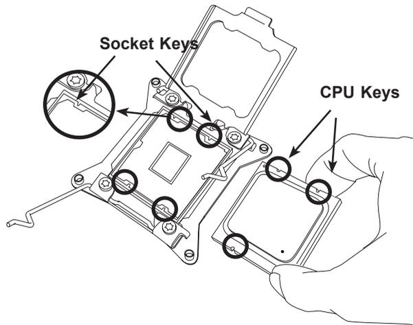
6. Once they are aligned, carefully lower the CPU straight down into the socket. To avoid damaging the CPU or socket, do not drop the CPU onto the socket, move it horizontally or vertically, or rub it against the socket pins.
