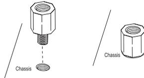
2. Locate the matching mounting holes on the chassis. Align the mounting holes on the motherboard against the mounting holes on the chassis.
