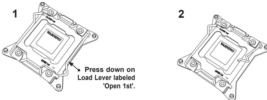
2. Press the second load lever labeled "Close 1st" to release the load plate that covers the CPU socket from its locking position.
