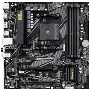
B550M DS3H AC R2 Motherboard - AMD Ryzen 5000 CPUs, 5+3 Phases VRM, up to 4733MHz DDR4 (O.C.), 1xPCIe 4.0 + 1xPCIe 3.0 M.2, Wi-Fi 5, 1GbE LAN, USB 3.2 Gen 1
