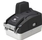
Canon imageFORMULA CR-L1. Maximum scan size: 108 x 228 mm, Optical scanning resolution: 300 x 300 DPI, Output colour depth: 24 bit. Product colour: Black, Grey. Sensor type: CMOS CIS, Daily duty cycle (max): 3000 pages, Light source: RGB LED. Auto document feeder (ADF) input capacity: 50 sheets. Media thickness (min): 0.08 mm, Card thickness (max): 0.2 mm, Auto Document Feeder (ADF) media weight: 64 - 157 g/m<sup>2</sup>
