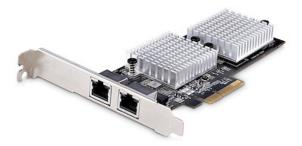
Install this 2-port 10GbE PCI Express (PCIe) Network Interface Card (NIC) into a server or computer to enable fast network speeds and enhanced network functionality by providing failover and redundancy protection to mission-critical servers/applications.
