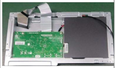
Tear out connect in red, remove the Mylar
