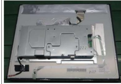
S7. Remove the Mylar of Power Board
