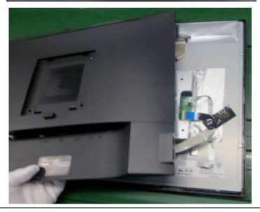
Tear down black tape then release the USB cable in red, you can take out rear cover.
