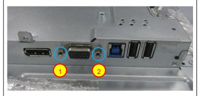
Use a hex screwdriver to remove 2 screws for unlocking mainboard
