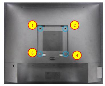
Use a Philips-head screwdriver to remove 4 screws for unlocking mechanisms.
