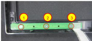
Use a Philips-head screwdriver to screw 3 screws for tighten key board (No.1~3 screw size=M2x2.5; Torque=0.9±0.4kgf.cm)
