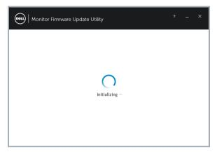
**3** The utility will load the firmware file automatically. Or, you can select your file manually by clicking ... and navigating to the UPG firmware file.
