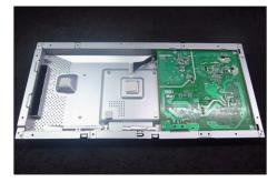
Take 1pcs interface board and 1pcs TBT board, then put plug the TBT board to the connector of the interface board. Take 1pcs MCU cable to connect the interface board with the TBT board. Use a Philips-head screwdriver to tighten 3pcs screws for locking the TBT board with interface board.
