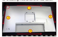
S4 Lift the rear cover up carefully. Disconnect the joystick key cable from the connector of the interface board, and then remove the rear cover and put it aside for later disassembling.
