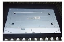
Move the bracket chassis module close to the panel, then connect the EDP cable to the connector of the panel, then turn over the bracket chassis and put it on the back of the bracket chassis.
