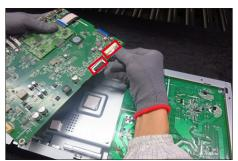
Turn over the interface board and locate the circuit boards and EDP cable into the bracket chassis. Use a Philips-head screwdriver to tighten 8pcs screws for locking the interface board and power board, then take 1pcs mylar sheet to insert the hooks of the bracket.
