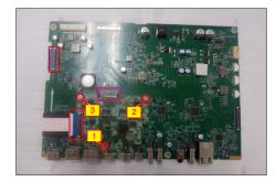
Take 1pcs EDP cable to connect with the interface board, and then connect the cable of power board to the connector of interface board.
