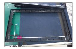
Move the middle bezel with the LED board close to the panel unit, then assemble the middle bezel with the front bezel and panel module.
