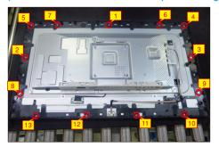
Disconnect the panel lamp and LED cable from the connectors, then release the panel lamp cable from the hook of the middle bezel.
