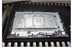
Take 1pcs IO cover to locate the hooks of the bracket chassis module as the picture below shown.
