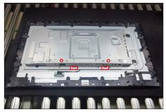
Lift up and take away the middle bezel, and put it on a cushion foam, and then tear off the mylar tape and adhesive tape on cable for releasing the LED board from the hook of the middle bezel.
