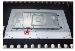
Adjust the bracket chassis, and then use a Philipshead screwdriver to tighten 4pcs screws for locking the bracket chassis with the panel.
