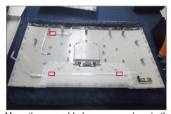
Move the assembled rear cover close to the panel unit, then connect the joystick key cable and sensor cable to the connectors of interface board. Put down the rear cover and push the rear cover on the positions marked for mechanisms engagement.
