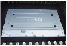
S14 Remove the Mylar tape from the hooks of the bracket.
