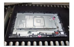
Use a Philips-head screwdriver to tighten 13pcs screws for locking the middle bezel with the panel module.
