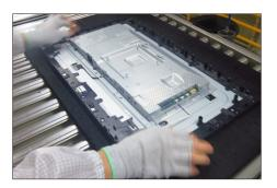
Connect the LED cable to the connectors of the board. Take 1pcs I/O cover to assemble with the bracket chassis.
