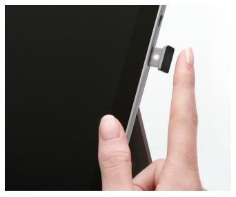
Match-in-Sensor™ Fingerprint Technology — Exceeds industry standards for False Rejection Rate (FRR 2%) and False Acceptance Rate (FAR 0.001%). Fingerprint data is secured in the sensor, so only an encrypted match result is transferred; versus match-on-host, where unsecured fingerprint data is transferred.
