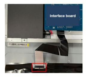
Unlock 13 screws to disassemble "Middle Frame" from "Panel"
