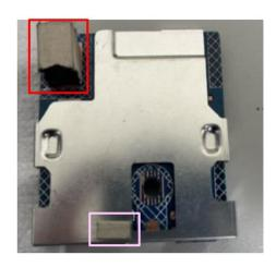
S11 Disassemble "USB board" from "USB Shielding"
