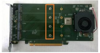
Step 3. The SSDs should be installed from top to bottom. To begin, remove the top screw.
