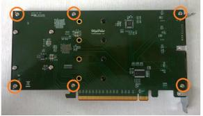
After removing the screws, carefully remove the front panel from the SSD7101A-1.
