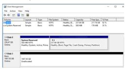
Create and format the partition using Disk Management to start using the SSD7101A-1 drive
