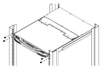
After the front brackets are secured, tighten all the screws.
